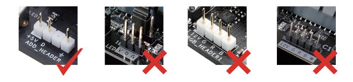
AEOLUS M3-1201 only support 5V addressable (digital) RGB header Manual is for reference only. Actual product may vary. The design of male and female motherboard sync connectors to deal with insufficient 5V socket
