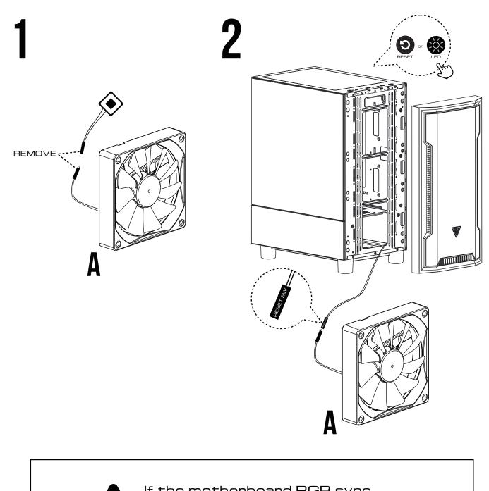
If the motherboard RGB sync function is used, the button function will be automatically disabled.
