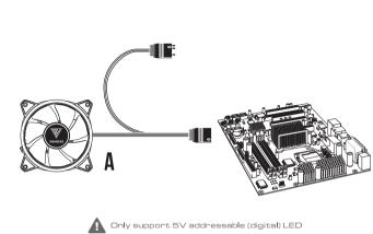
The design of male and female motherboard sync connectors to deal with insufficient 5V socket
