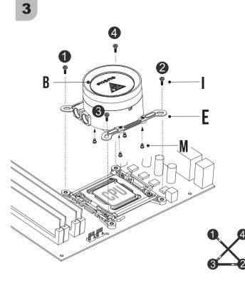
A Please tighten the screws in a diagonal sequence to spread the tension properly.
